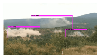
Fig. 6. Prediction result of the YOLOv4 after the training. We can see that the YOLOv4 model can correctly detect and label smoke in images.
