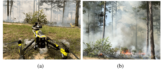
Fig. 1. Deploying a UAS with both vision and olfaction sensors in a prescribed burn to monitor wildfires. (a) The UAS is ready to take off and (b) the UAS is flying above the burning area to collect air quality and meteorological data. These images were taken from the prescribed burn conducted in May 2022.
