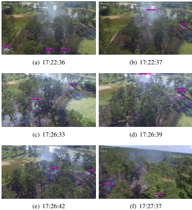
Fig. 10. Smoke prediction generated by the trained YOLOv4 model. Images were captured from the UAS during the flight at different times. Red squares in the images highlighted the detected smoke areas. High resolution images can be found via this link [49].
